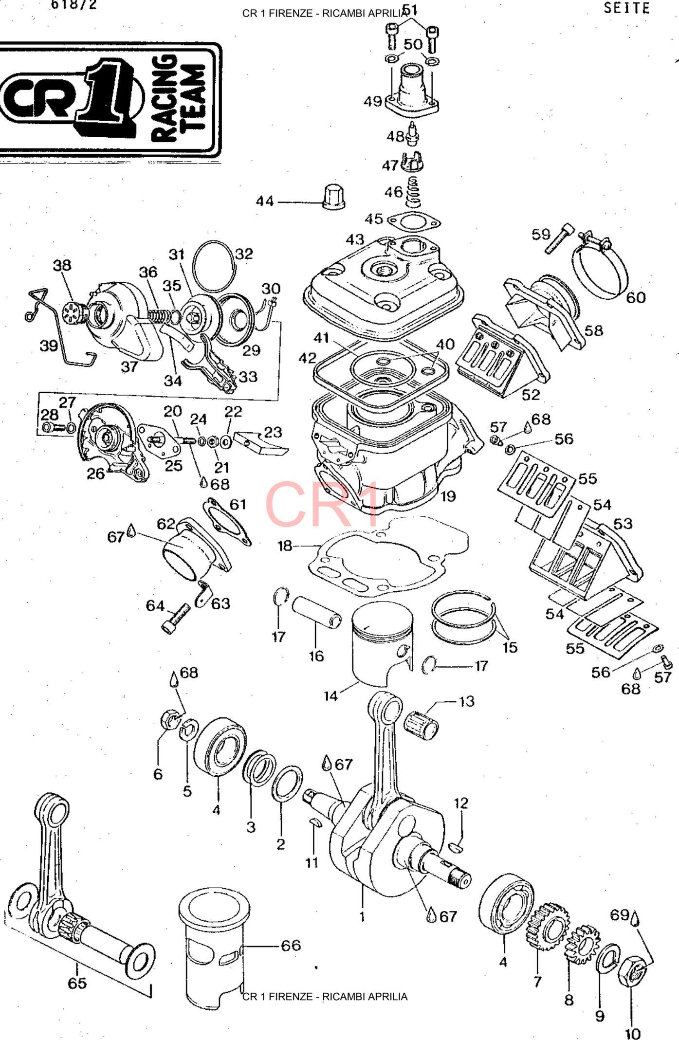
KURBELWELLE, KOLBEN, ZYLINDER, ZYLINDERKOPF;
